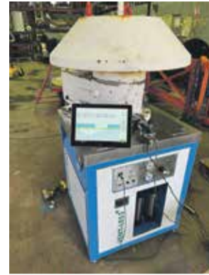
Vent-Less at a customer's site, testing a breather valve
